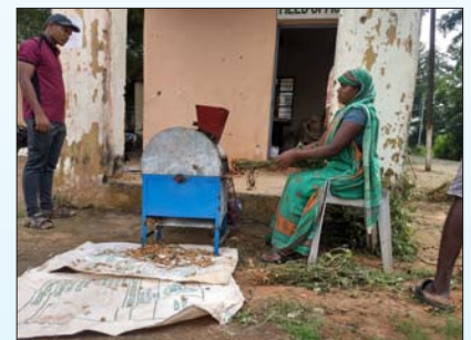
Stripping of the pods with developed power operated groundnut stripper
