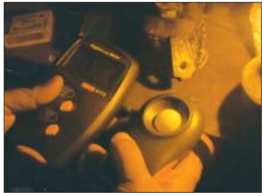
Measuring Illumination level
