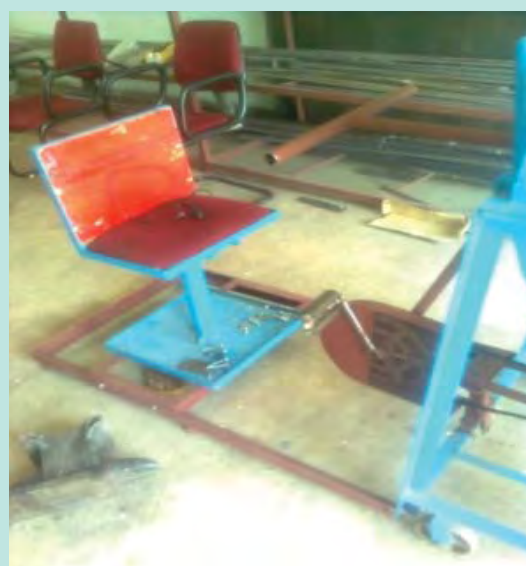
Fig. 53-54. Riding and sitting type pedalling system in DRWA maize dehusker-sheller
