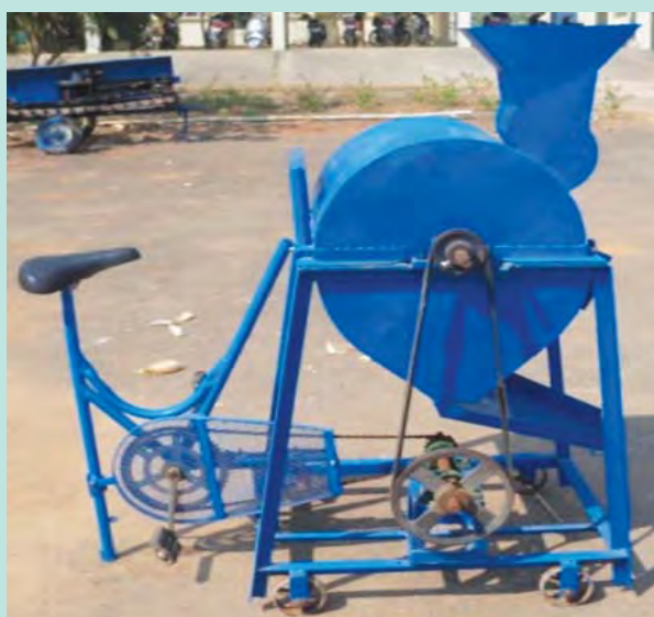
Fig. 53-54. Riding and sitting type pedalling system in DRWA maize dehusker-sheller
