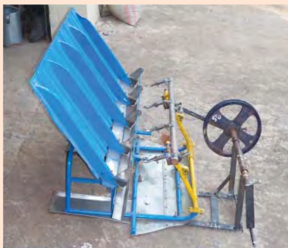
Fig. 52. Side View of a Mechanism for Plucking Arm & Finger for Powering
