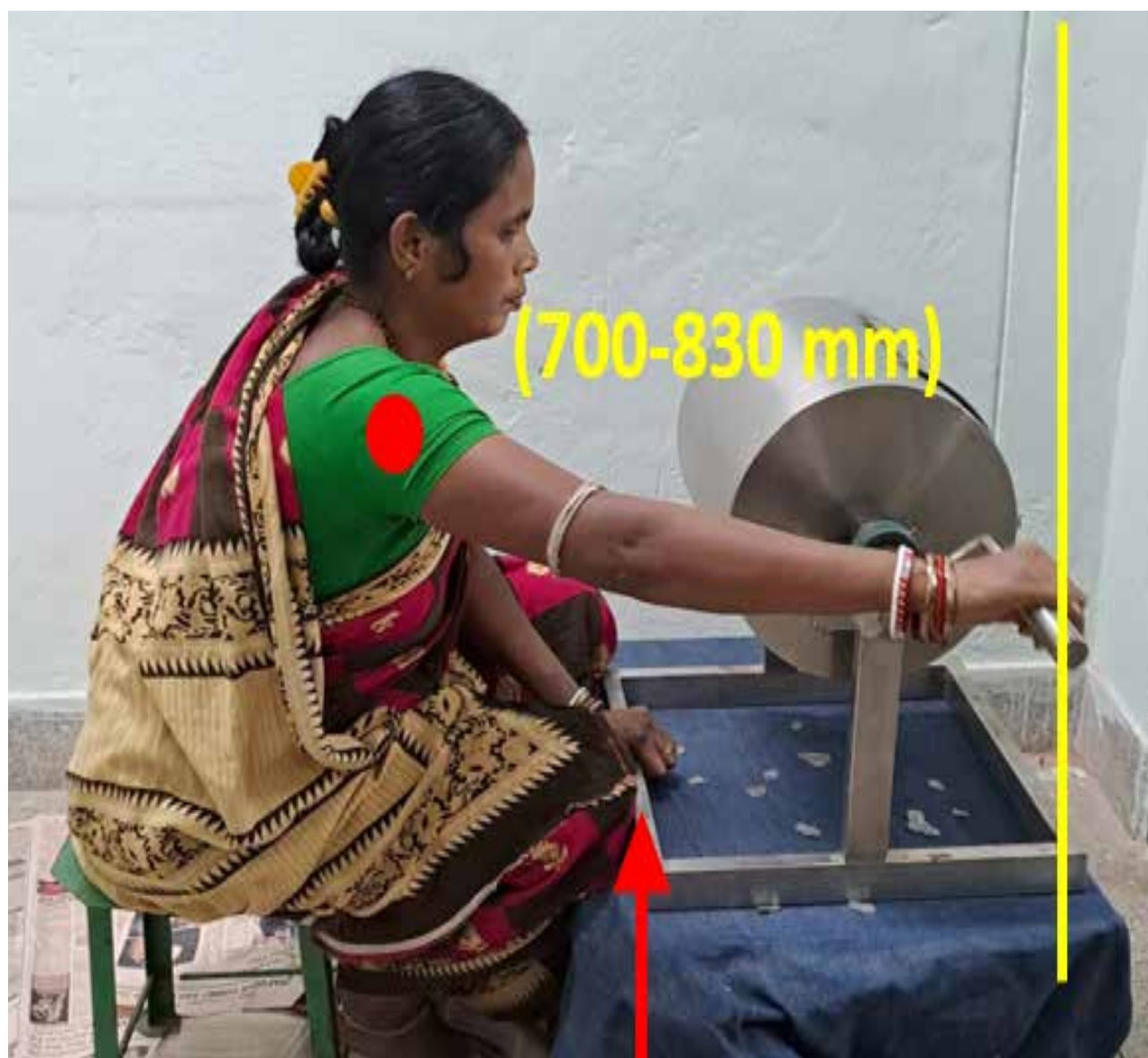
Fig. 2.50 Design consideration for CIFT manually operated fish descaler
