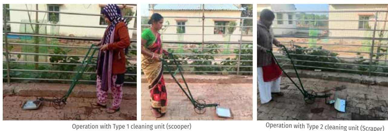
Fig. 2.53 Operation with Type 1 cleaning unit (Scooper) & Type 2 cleaning unit (Scraper)
