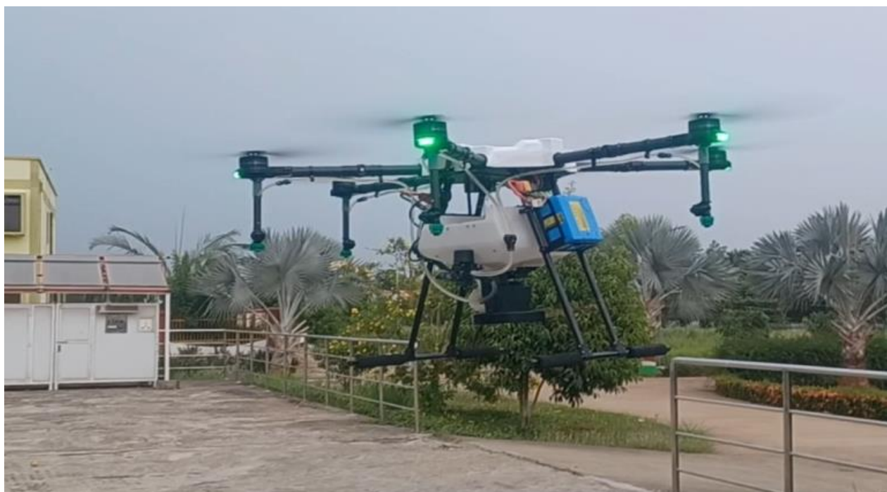
Fish feed dispersion by using drone-based seed broadcaster
