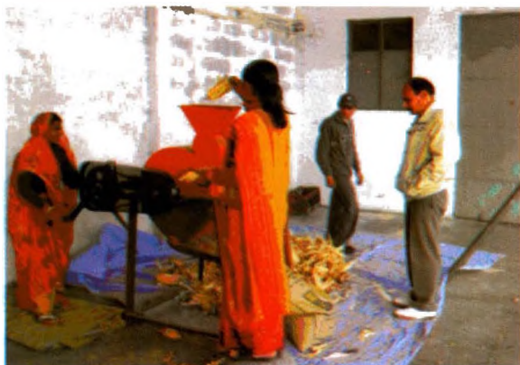
Farmwomen operating the prototype with modified cylinder in standing posture
