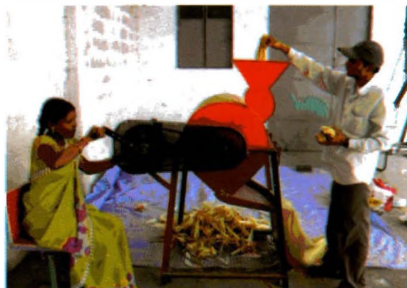
Farmwomen operating the prototype with modified cylinder in sitting posture
